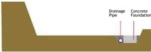
Foundation of the reinforced wall
