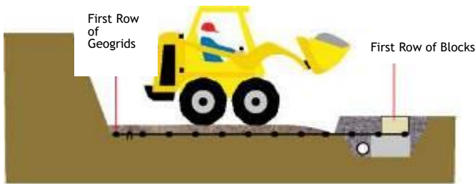
Laying the first row of geogrid and placing the blocks for the reinforced walls
